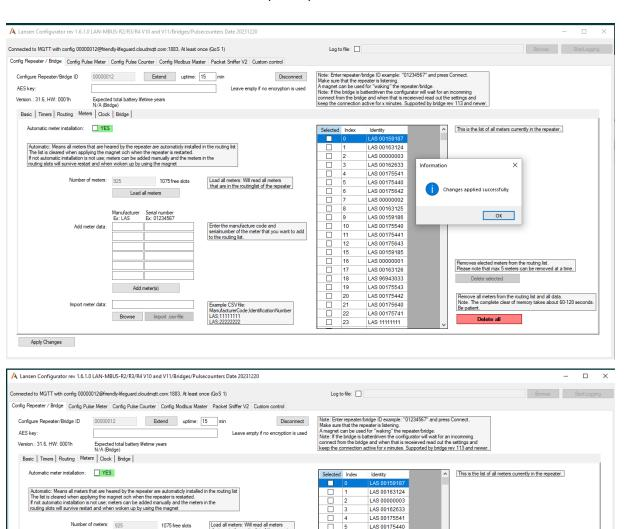
Enter the manufacture code and serialnumber of the meter that you want to add to the routing list. LAS 00000002 LAS 00163125 LAS 00159186
