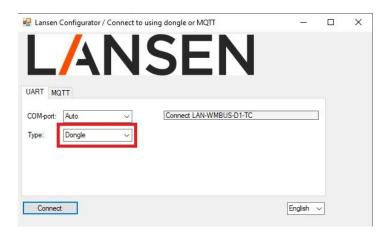
To change the settings to the gateway one must first connect to the gateway. This is done by putting in the serial number which can be found on the poke protection or the front label on the device, then clicking 'Connect'. Once you have connected to the device you can change all the settings and parameters. The packet sniffer will not be operating when connected through wire.
