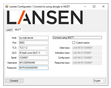
If everything works, then you are now connected to the MQTT server. In the example below, connection has been made with serial number 0000012 to the MQTT server friendly-lifeguard.cloudmqtt.com.
