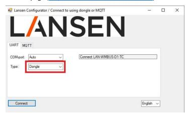
The below window is shown once the connection to the dongle is successful.
