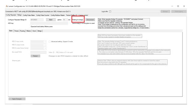
Once the gateway is connected to the MQTT server and connection is established by Lansen Configurator, the countdown of the uptime will start. The counter shows the time left before the gateway shuts down the connection with the MQTT server.
