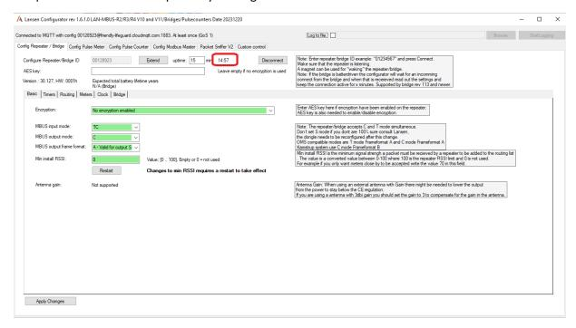
The gateway closes the connection when the timer reaches 00:00 or when the button *Disconnect* is clicked.
