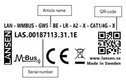
Article name: Full article name code of the device. QR-code: Includes the wM-Bus serial number of the device. Serial number: Full device information (example above:
